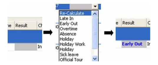
Note: After correcting report data, you should press **Update Report** button without checking on 'Rebuild All'. If you check on 'Rebuild All', T/A data will return to the original data before such correction.
