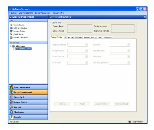
Select Search Device menu, click Search BioEntry, select either serial port or TCP/PI and then press search button. If device is found as a result of search, result report reading '--- device(s) found' is shown. Press OK button to select device.
