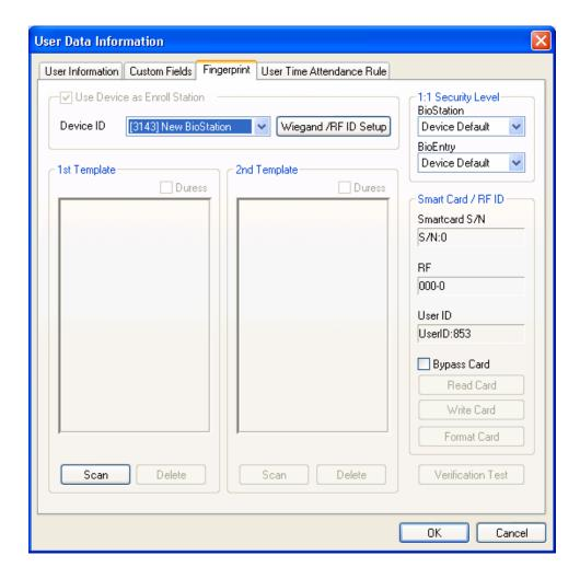
Acquire first template by pressing the Scan button followed by touching a finger on the USB fingerprint scanner twice.
