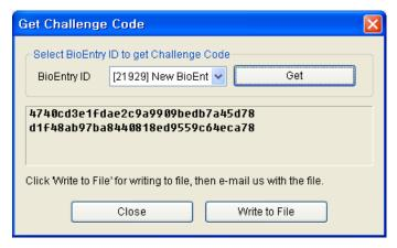
The support team will send you the unlock code file corresponding to the challenge code. Use Unlock a BioEntry and Password to the Default button to resolve the device. Then, the device is unlocked and password is changed to default (null).
