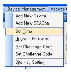
• You can synchronize the time of all of the networked BioEntry™ to the time of host PC. If you already checked on the Synchronize current PC time at startup check box, which is on Options → Preference → Device Time Setting, you do not need to synchronize the time on this menu.
