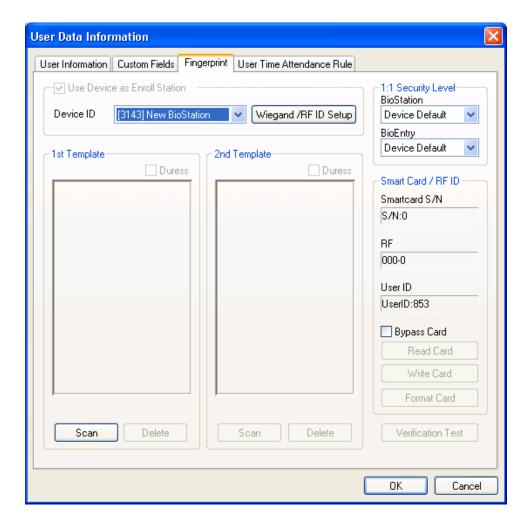
• In case of stand alone mode without USB scanner, check Use BioStation as Enroll Station, press scan button, place a finger twice on device and then input the first fingerprint information. In case that device is configured by 2 or more networks, specify BioStation ID, press scan button, place a finger on device twice and then input the first fingerprint information.
