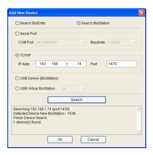
Administrator needs to know IP address and port # (1470). Once device is connected properly, IP address is displayed as one group and device ID is displayed with a bracket [\*\*\*\*] on device tree window.
