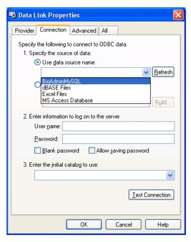
Enter the ID and password of the DB server. It there is no password designated, check on the Blank password. If there is any password, check on the Allow saving password.
