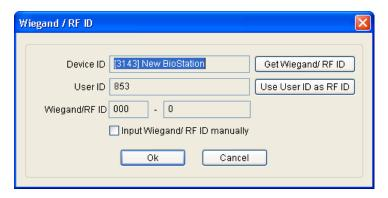
If you use BioStation RF or use the normal BioStation along with an external Wiegnad card reader, you need to allocate the card ID to each user. Press this button to designate the users' card ID.
