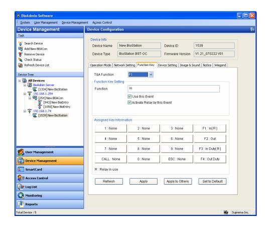
Set 16 keys in device and choose one out of 16 function keys to check function key event message displayed on BioStation LCD, use of this function key and relay use.
