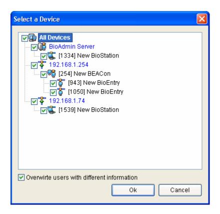
**Transfer checked users to device** is to transfer user DB in host PC to device. To run a device, user data including fingerprint information should be transferred to device after user enrollment.
