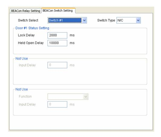
Select a switch to set up the configuration. Once you select a switch, applicable items for the selected switch will be activated on the switch setting window.
