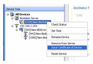
To communicate with the BioStation, select the unauthorized BioStation and press the right button of the mouse. Press **Issue Certificate of Device** menu. After issuing the certificate, you can use this BioStation.
