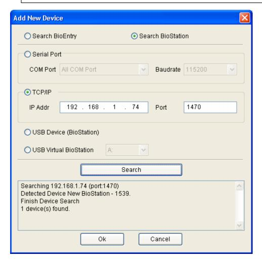
Once it's connected to device successfully, new device ID and network connected to device are also displayed in device tree window.
