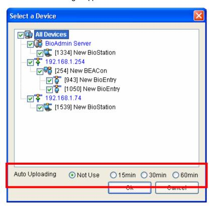
Once auto uploading is applied, **status**: **auto uploading on** is indicated on task box.
